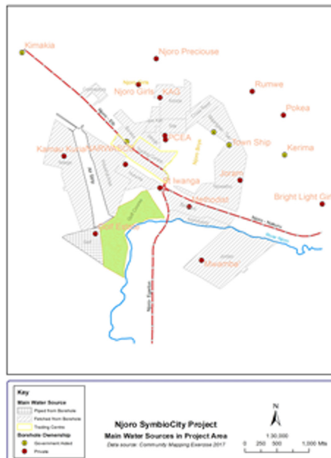
A Map showing location of borehole water sources in the project area
